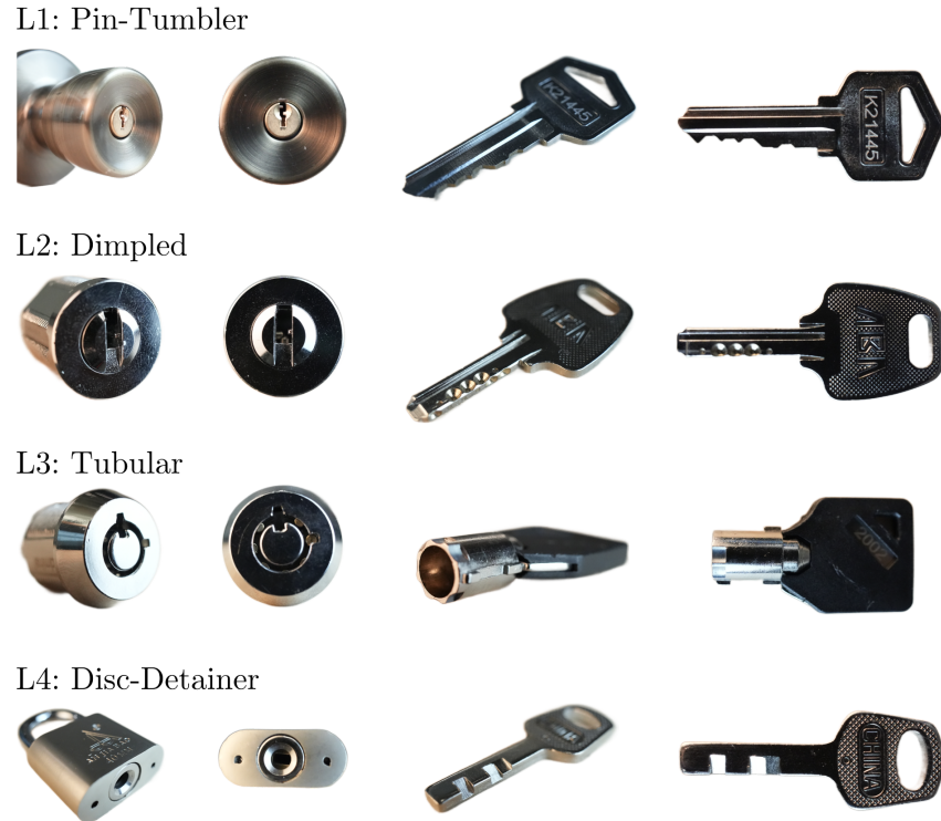
Figure 4.5: The four types of key and lock pairs tested. L1 is a common pin-tumbler lock used on front doors. L2 is a dimpled cam lock that uses pin-tumblers like L1, but they also press on the sides of the key into the dimples. L3 is a tubular lock with a circular shape that must be pressed into the lock’s circular opening. L4 is a disc-detainer which features rotating discs inside the lock that must be aligned.
